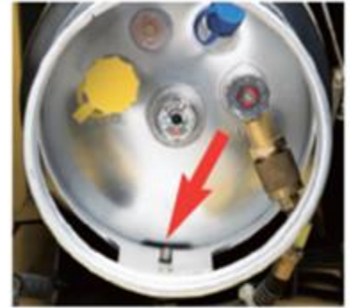
3. Place the bracket locator pin in the cylinder locator hole.
