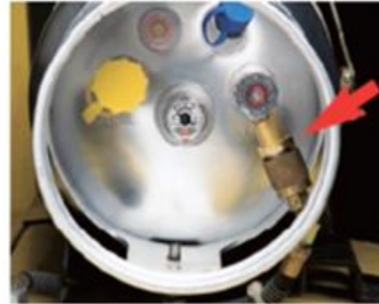
5. Connect propane fitting until it is firmly connected, leak free (no tools required). Open valve and start engine.
