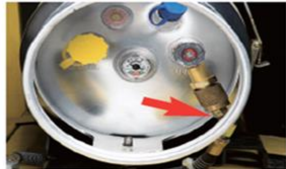
5. Connect propane fitting until it is firmly connected, leak free (no tools required). Open valve and start engine.
