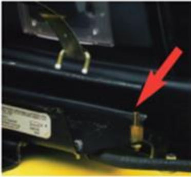
1. Find the locator pin on the bracket.
